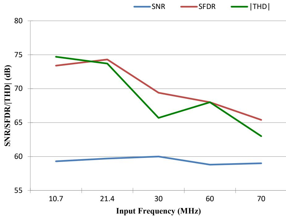
Figure 24: SNR/THD/SFDR vs.  $F_{IN}$ ,  $F_s = 100$  MHz
