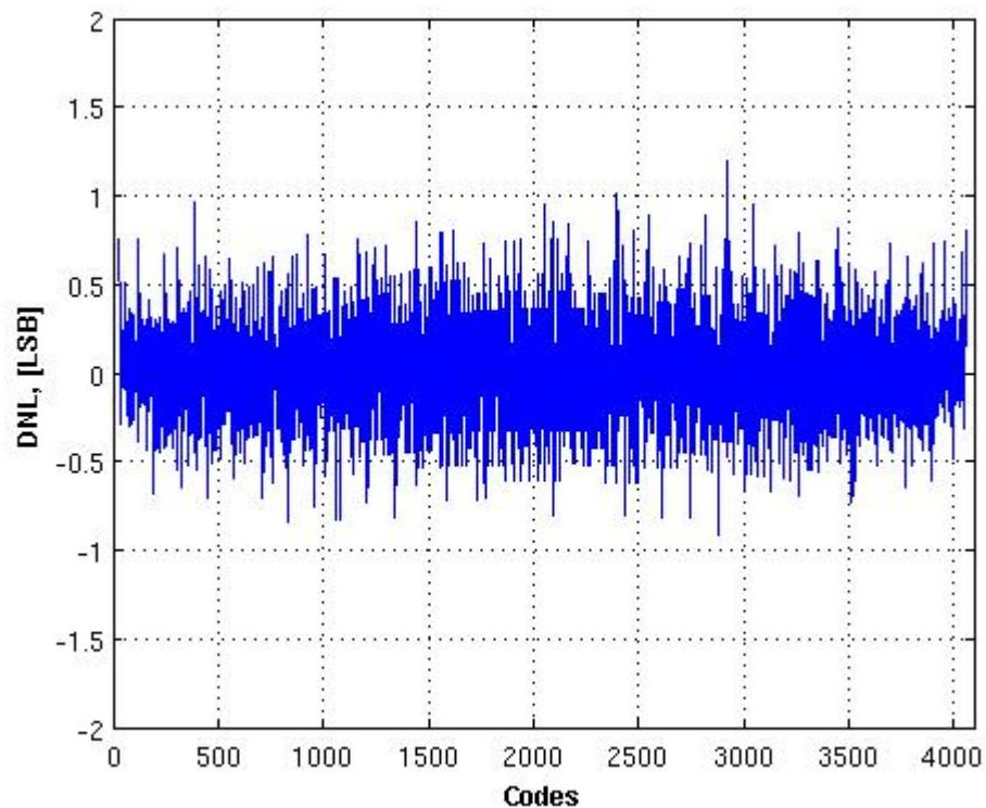
Figure 32: Differential nonlinearity (DNL),  $F_{IN} = 10.7$  MHz,  $F_S = 100$  MHz
