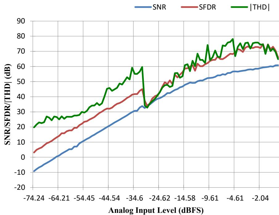
Figure 25: SNR/THD/SFDR vs. analog input level,  $F_{IN} = 10.7$  MHz,  $F_S = 100$  MHz
