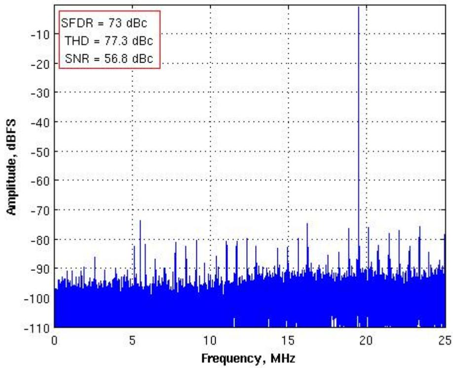
Figure 7: Single-Tone FFT with  $F_{IN} = 30.9$  MHz,  $F_S = 50$  MHz,
