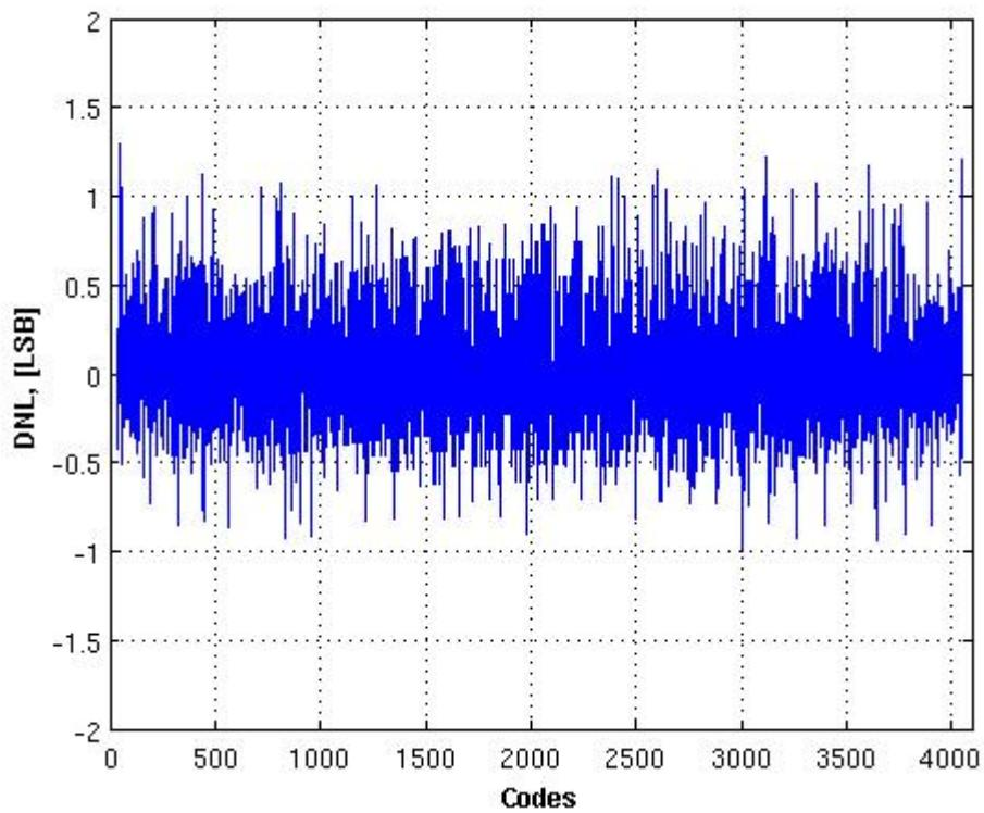
Figure 18: Differential nonlinearity (DNL),  $F_{IN} = 10.7$  MHz,  $F_s = 50$  MHz
