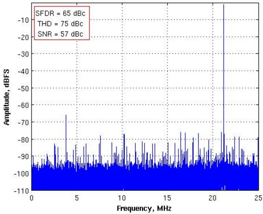
Figure 9: Single-Tone FFT with  $F_{IN} = 70.6$  MHz,  $F_S = 50$  MHz,
