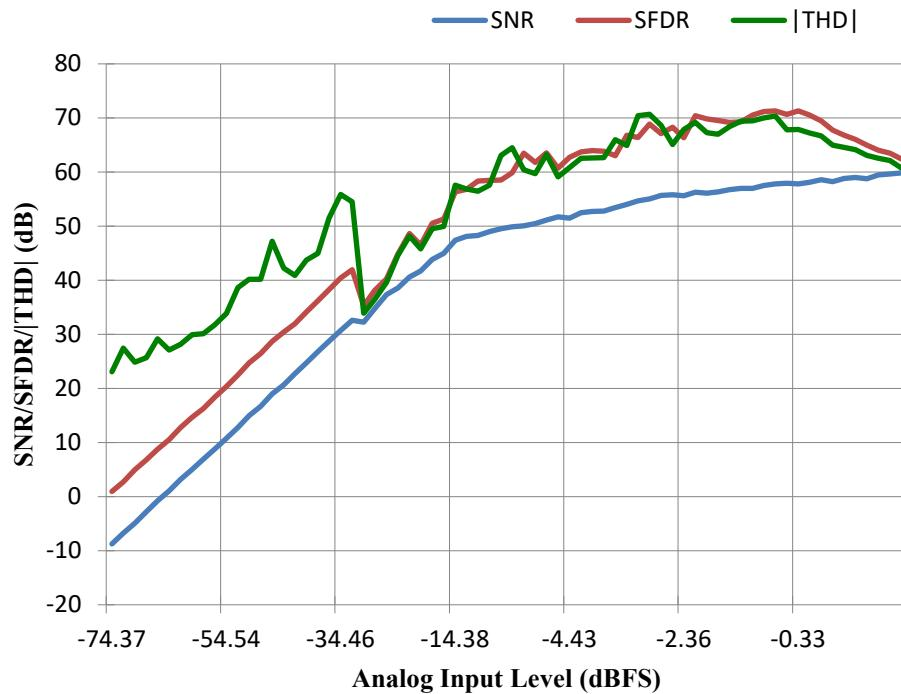
Figure 36: SNR/SFDR/|THD| vs. analog input level,  $F_{IN} = 21.4$  MHz,  $F_s = 125$  MHz
