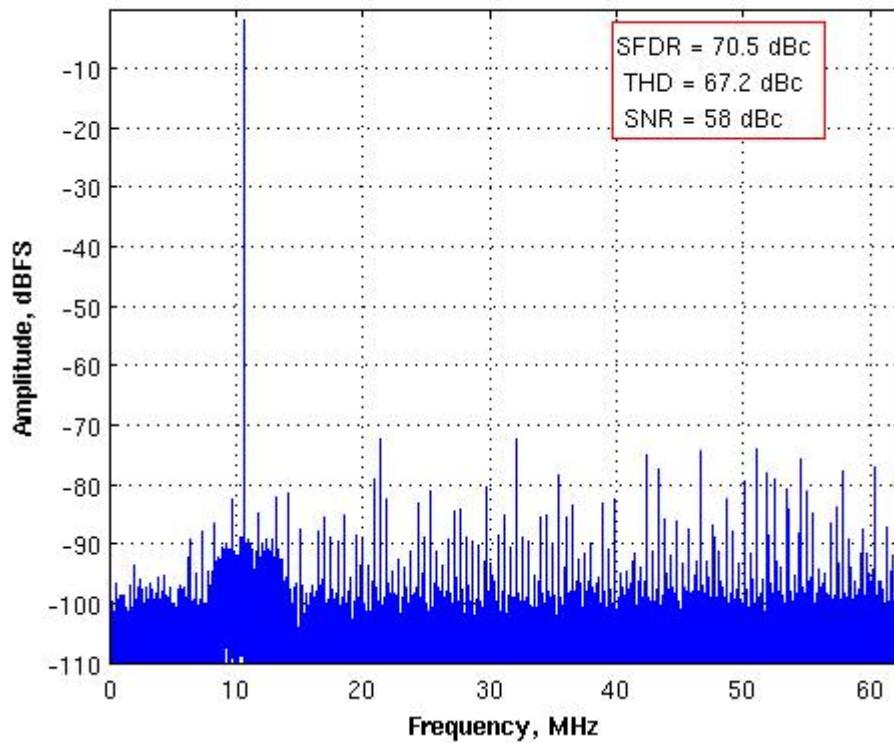
Figure 33: Single-tone FFT with  $F_{IN} = 10.7$  MHz,  $F_s = 125$  MHz,
