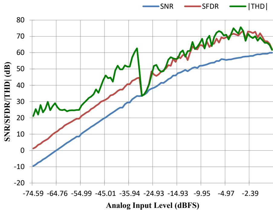
Figure 26: SNR/THD/SFDR vs. analog input level,  $F_{IN} = 21.4$  MHz,  $F_S = 100$  MHz
