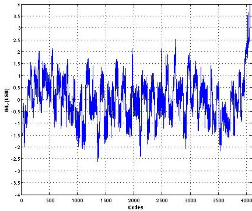
Figure 31: Integral nonlinearity (INL),  $F_{IN} = 10.7$  MHz,  $F_S = 100$  MHz
