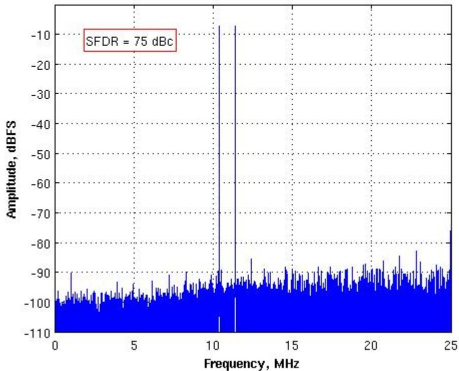
Figure 13: Two-Tone FFT with  $F_{IN1} = 10.2$  MHz,  $F_{IN2} = 11.2$  MHz,  $F_s = 50$  MHz,
