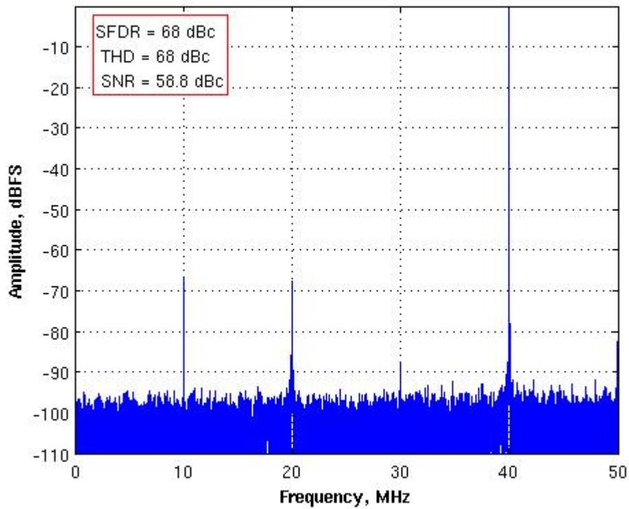
Figure 22: Single-tone FFT with  $F_{IN} = 60$  MHz,  $F_s = 100$  MHz,
