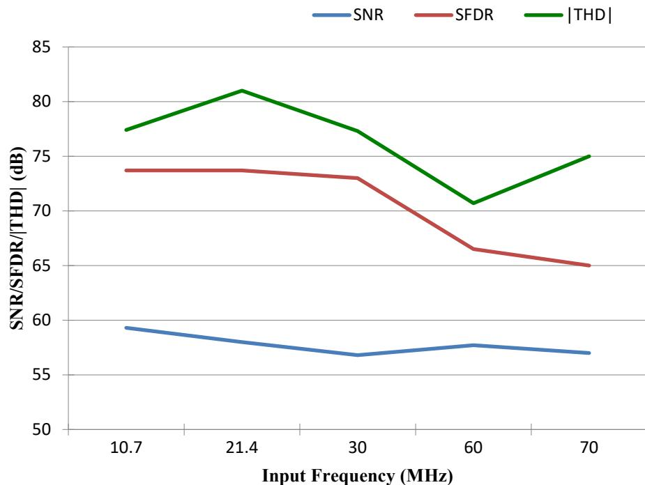
Figure 10: SNR/THD/SFDR vs.  $F_{IN}$ ,  $F_S = 50$  MHz,
