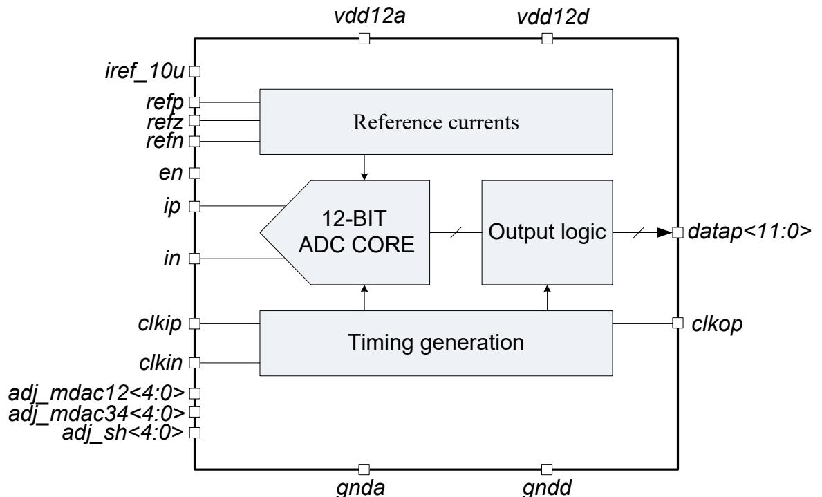
Figure 1: 12-bit 50/100/125 MSPS 1-channel ADC structure
