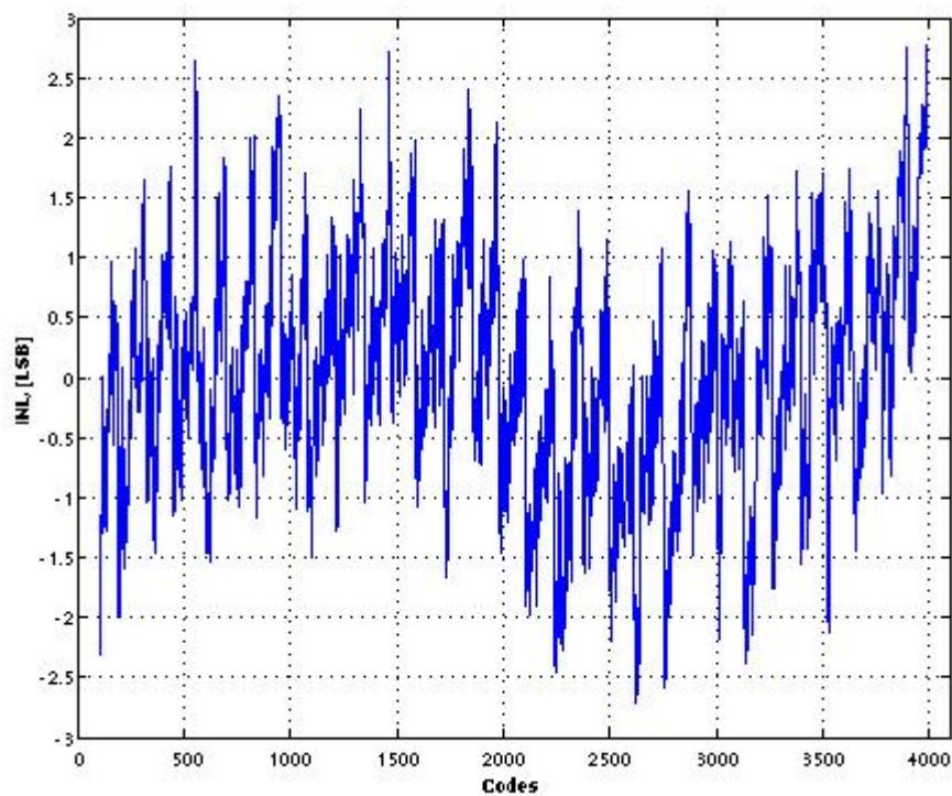
Figure 17: Integral nonlinearity (INL),  $F_{IN} = 10.7$  MHz,  $F_s = 50$  MHz
