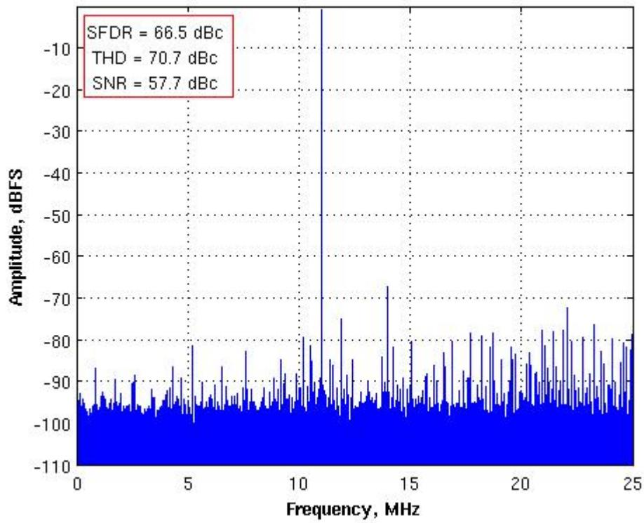
Figure 8: Single-Tone FFT with  $F_{IN} = 60.7$  MHz,  $F_S = 50$  MHz,
