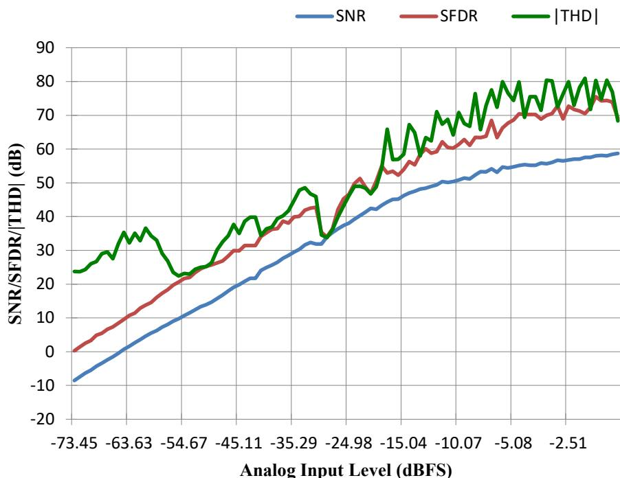
Figure 12: SNR/THD/SFDR vs. Analog Input Level,  $F_{IN} = 21.4$  MHz,  $F_S = 50$  MHz
