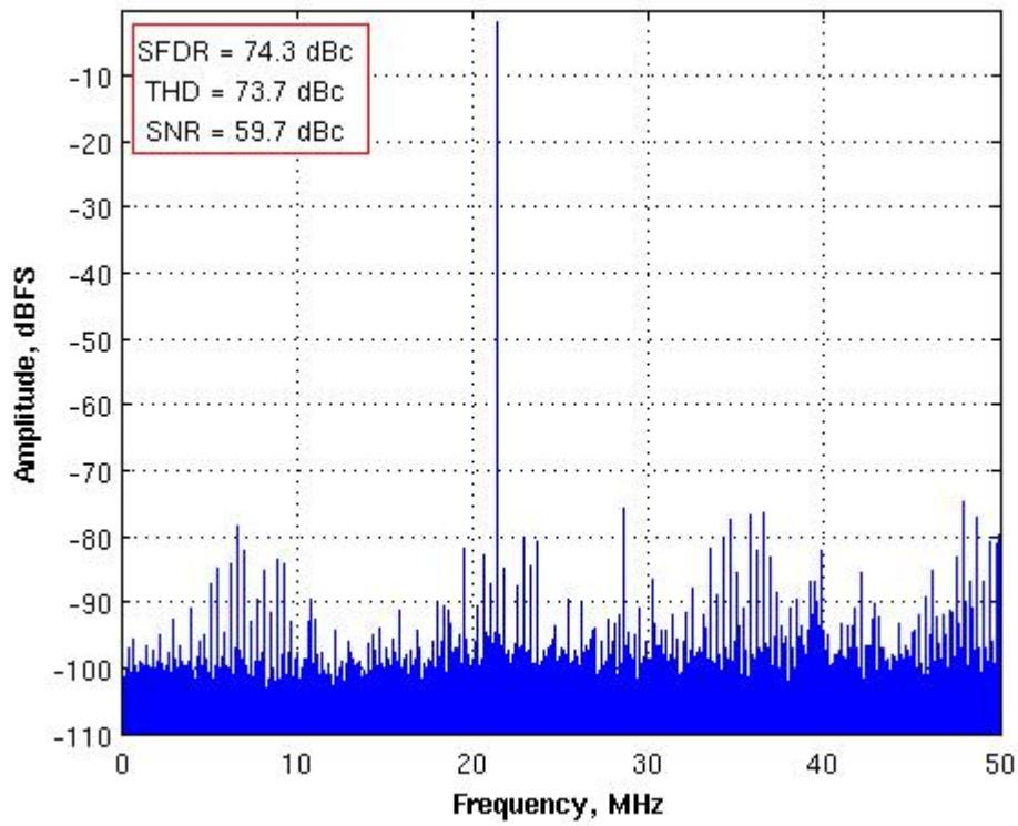
Figure 20: Single-Tone FFT with  $F_{IN} = 21.4$  MHz,  $F_s = 100$  MHz,
