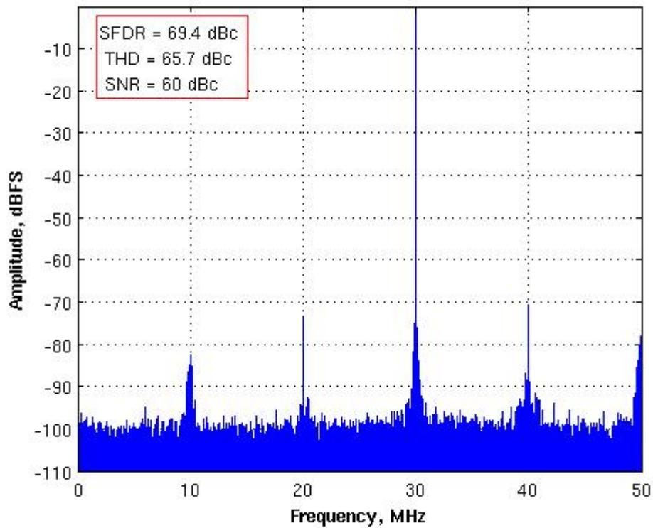
Figure 21: Single-tone FFT with  $F_{IN} = 30$  MHz,  $F_s = 100$  MHz,
