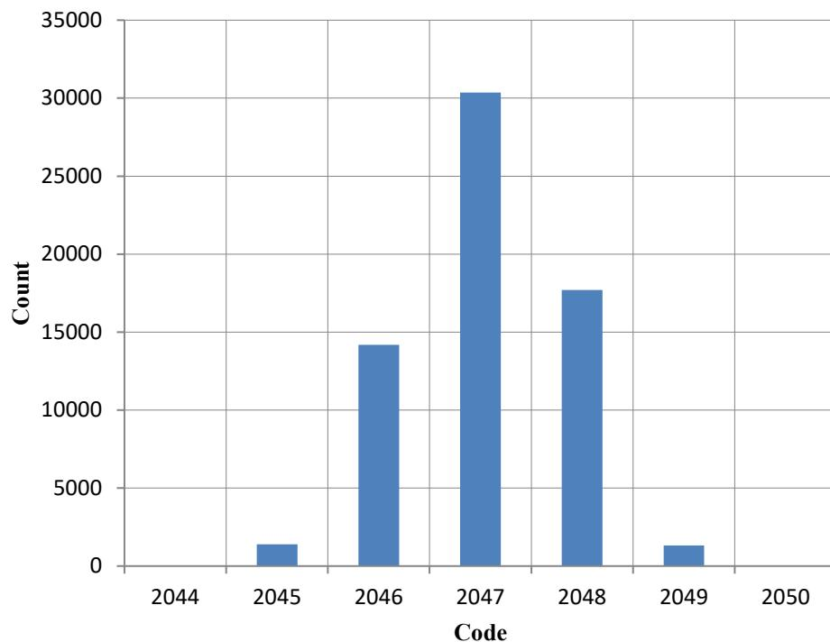
Figure 15: Grounded Input Histogram,  $F_s = 50$  MHz
