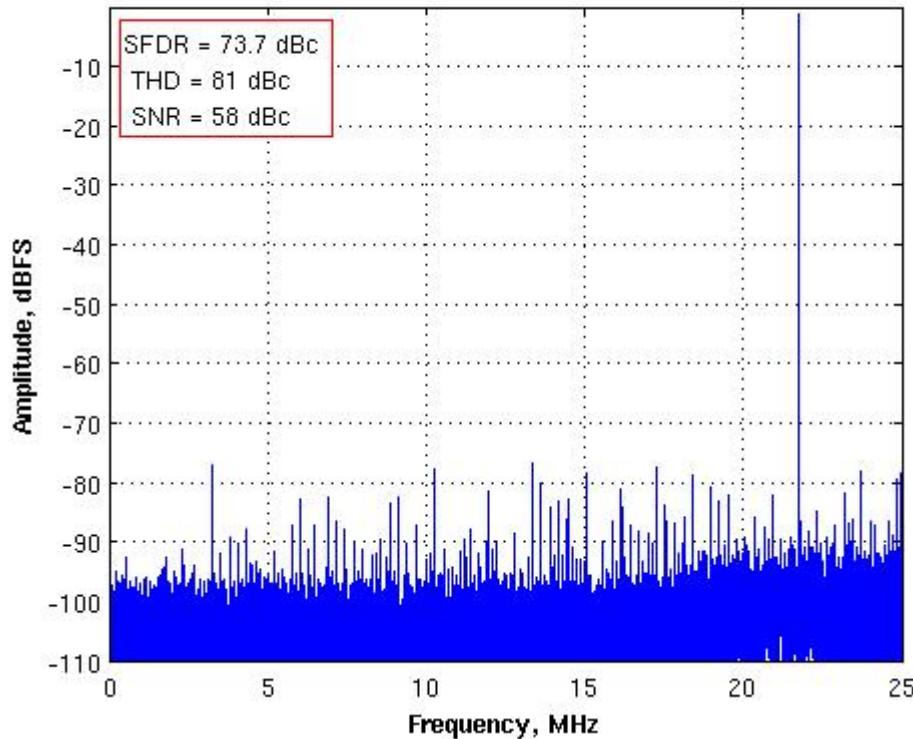
Figure 6: Single-Tone FFT with  $F_{IN} = 21.4$  MHz,  $F_S = 50$  MHz,
