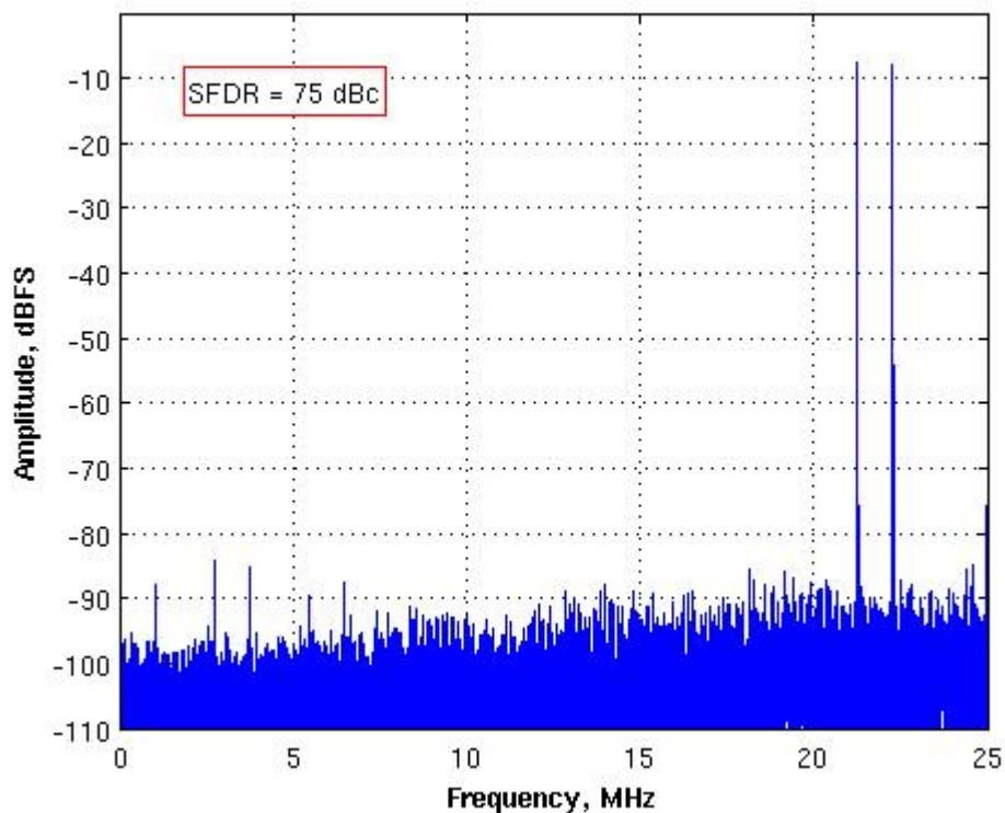
Figure 14: Two-Tone FFT with  $F_{IN1} = 20.9$  MHz,  $F_{IN2} = 21.9$  MHz,  $F_s = 50$  MHz,
