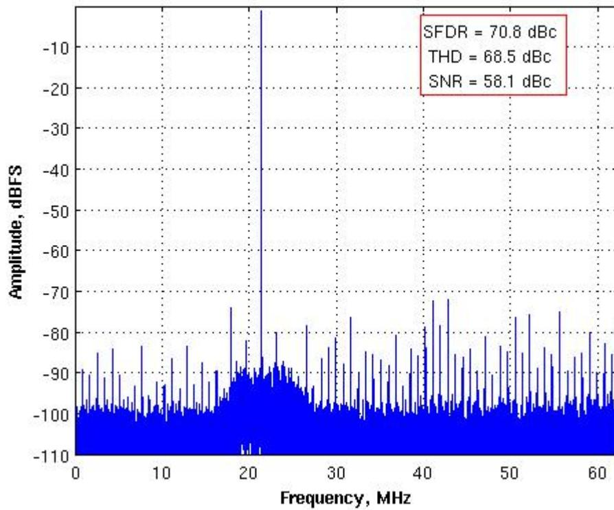
Figure 34: Single-tone FFT with  $F_{IN} = 21.4$  MHz,  $F_s = 125$  MHz,
