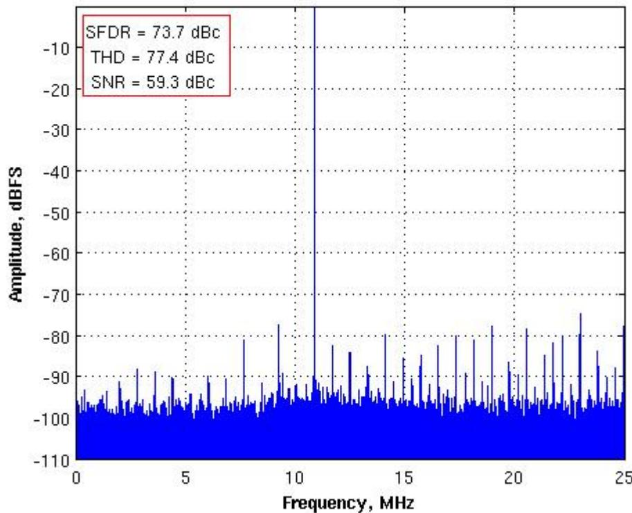
Figure 5: Single-Tone FFT with  $F_{IN} = 10.7$  MHz,  $F_S = 50$  MHz,
