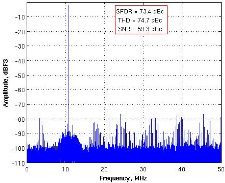
Figure 19: Single-tone FFT with  $F_{IN} = 10.7$  MHz,  $F_s = 100$  MHz,
