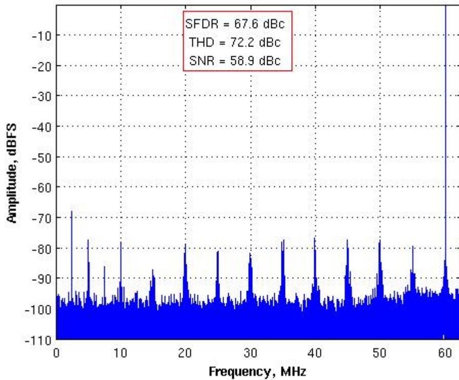
Figure 35: Single-tone FFT with  $F_{IN} = 60$  MHz,  $F_s = 125$  MHz,
