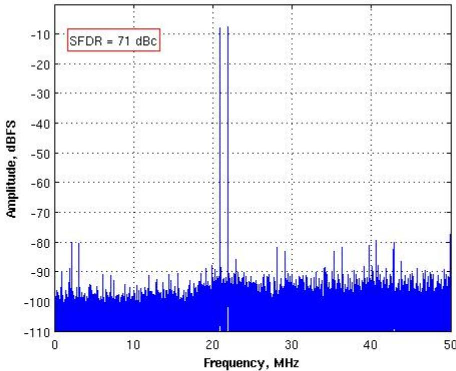
Figure 29: Two-tone FFT with  $F_{IN1} = 20.9$  MHz,  $F_{IN2} = 21.9$  MHz,  $F_S = 100$  MHz,
