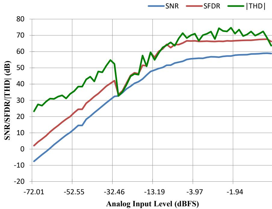
Figure 37: SNR/THD/SFDR vs. analog input level,  $F_{IN} = 60$  MHz,  $F_S = 125$  MHz
