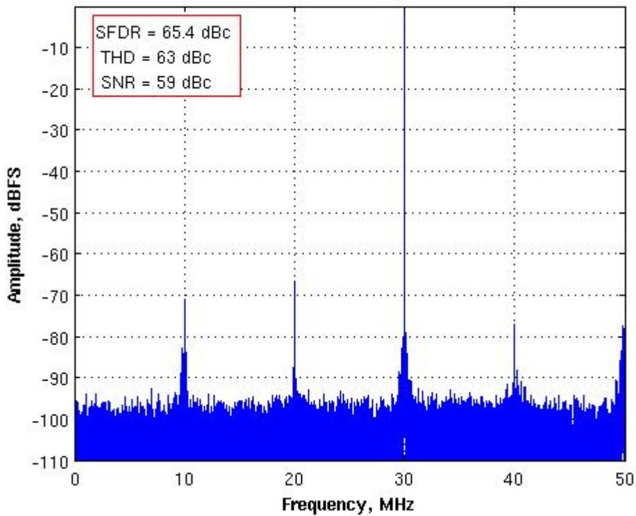
Figure 23: Single-tone FFT with  $F_{IN} = 70$  MHz,  $F_s = 100$  MHz,
