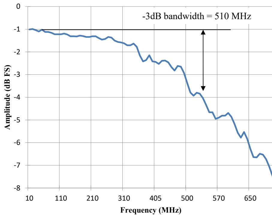
Figure 28: Full-power bandwidth vs. frequency,  $F_S = 100$  MHz
