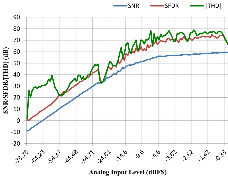
Figure 11: SNR/THD/SFDR vs. Analog Input Level,  $F_{IN} = 10.7$  MHz,  $F_S = 50$  MHz
