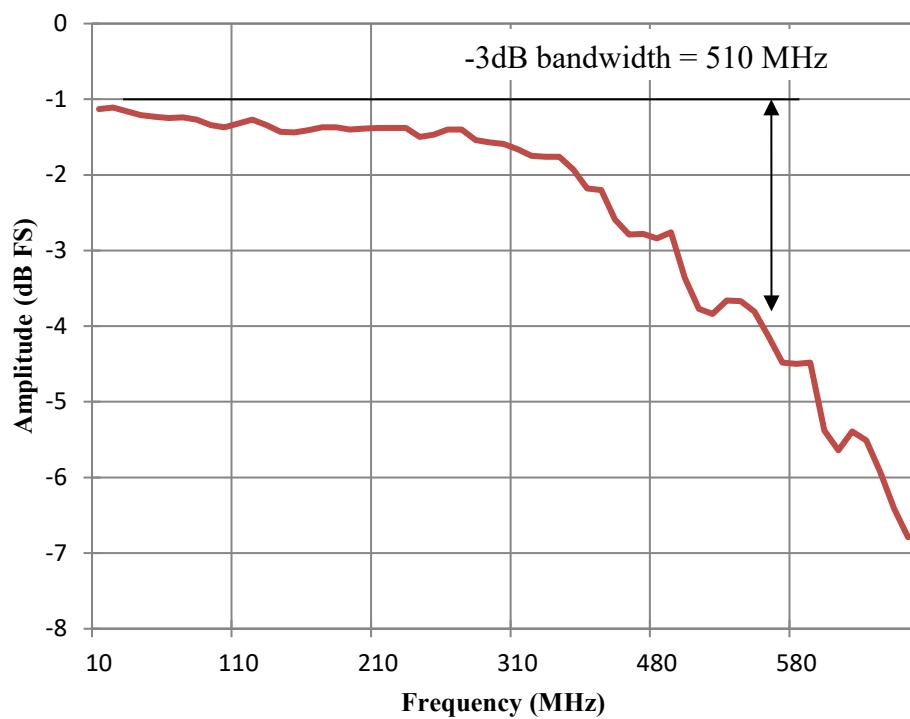
Figure 16: Full-power bandwidth vs. frequency,  $F_s = 50$  MHz
