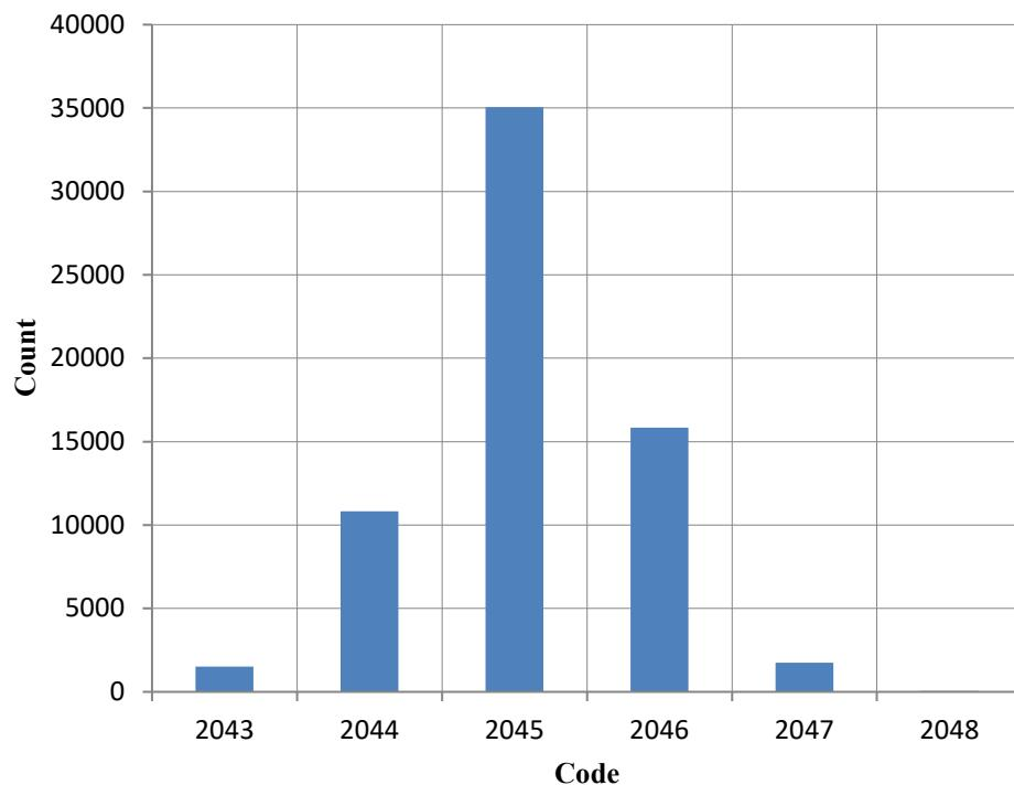
Figure 27: Grounded input histogram,  $F_S = 100$  MHz
