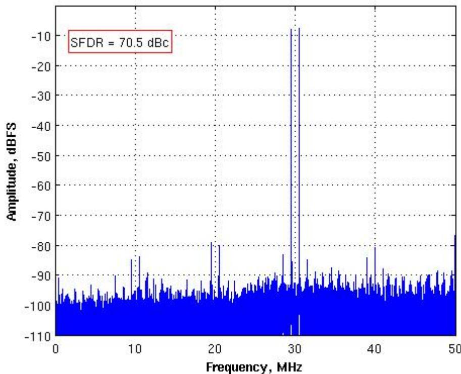
Figure 30: Two-tone FFT with  $F_{IN1} = 29.5$  MHz,  $F_{IN2} = 30.5$  MHz,  $F_S = 100$  MHz,
