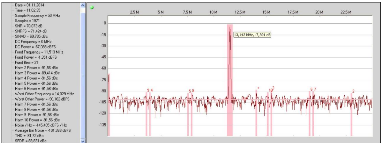
Figure 5: Spectrum, F_s = 50 MSPS, F_{in} = 11.513 MHz
