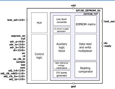
applications, requiring low power consumption and supply voltage. Data to be write are set at data input pin di<15:0>. Writing process starts, when signal wr goes to "1". Data di<15:0>, page address adr\_p<4:0>, word address in page adr\_w<2:0> are latched into internal registers and cannot be changed until the end of the writing process. At the end of the writing, the ready = "1" flag is set.
