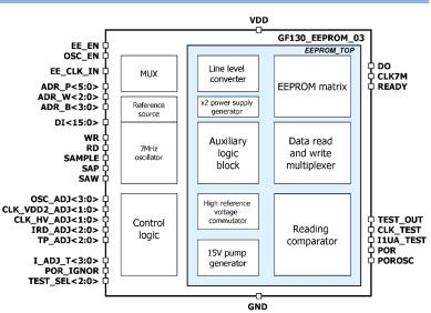
word ADR\_B<3:0>. After applying the reading strobe, the DO signal is set at the output corresponding to the reading data from the corresponding addresses of the EEPROM cell. EEPROM also has a 7MHz built-in oscillator. The oscillator has frequency control inputs to compensate for process variation. Memory is optimized for usage in the industrial and commercial applications, requiring low power consumption and supply voltage. Metal stack 6LM CU 1TM SP 9KA.
