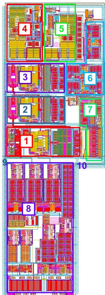
Figure 2: Intermediate-frequency amplifier layout
