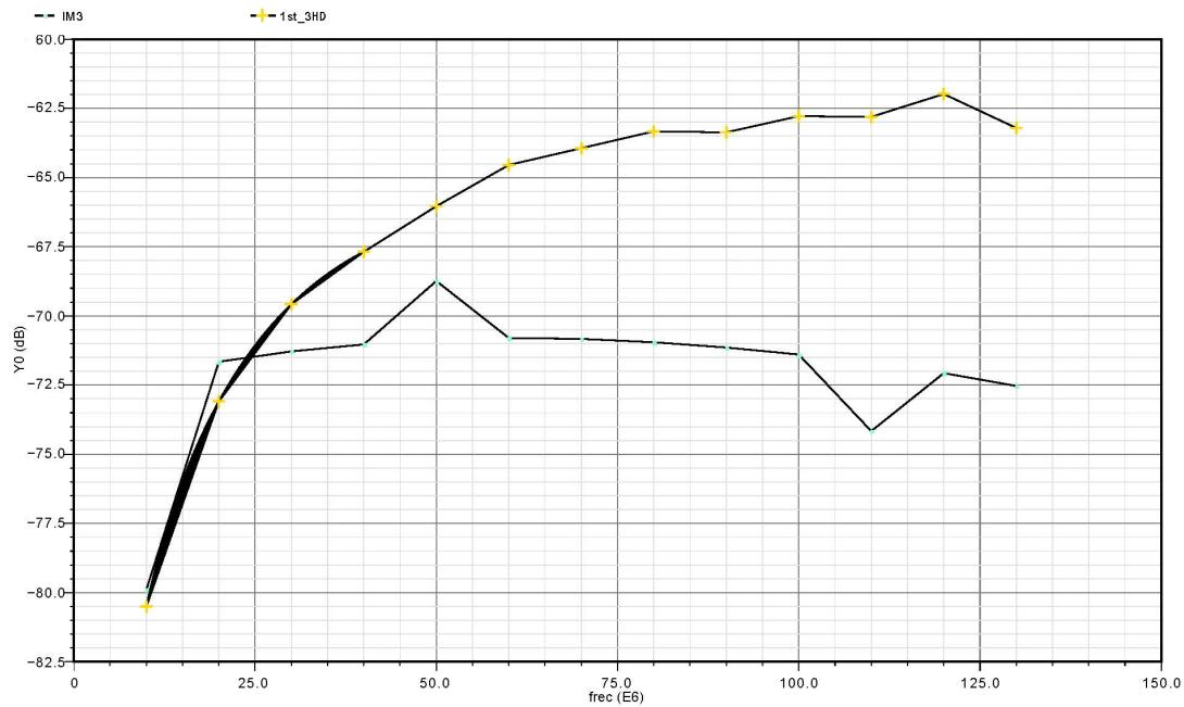
Figure 5: IM3 and HD3 (min gain, Vout=1V<sub>p-p</sub>)
