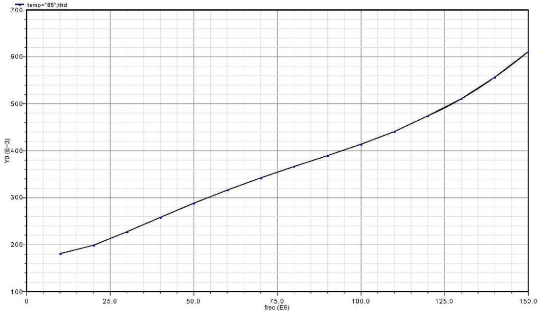
Figure 6: Thd (min gain, Vout=1V<sub>p-p</sub>)
