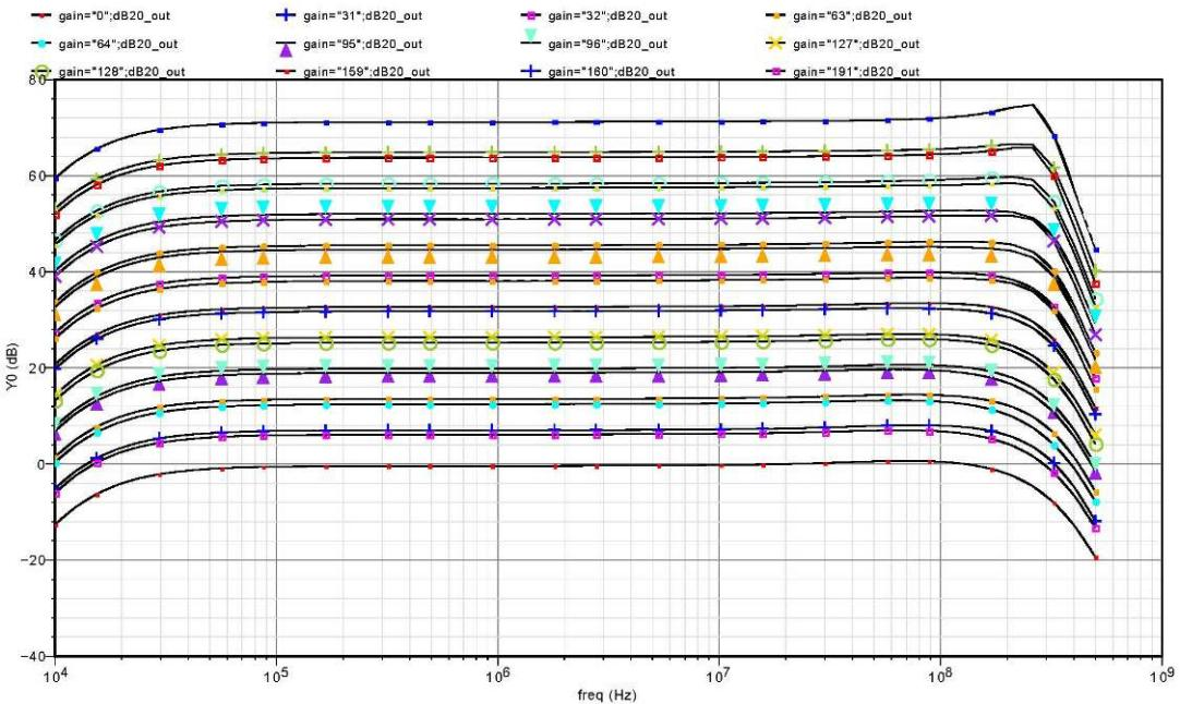
Figure 4: Amplitude frequency characteristics over gain code IFA
