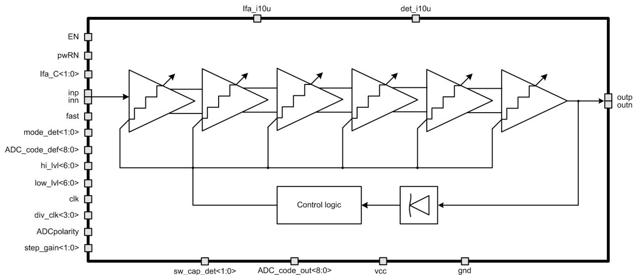
Figure 1: Intermediate-frequency amplifier structure
