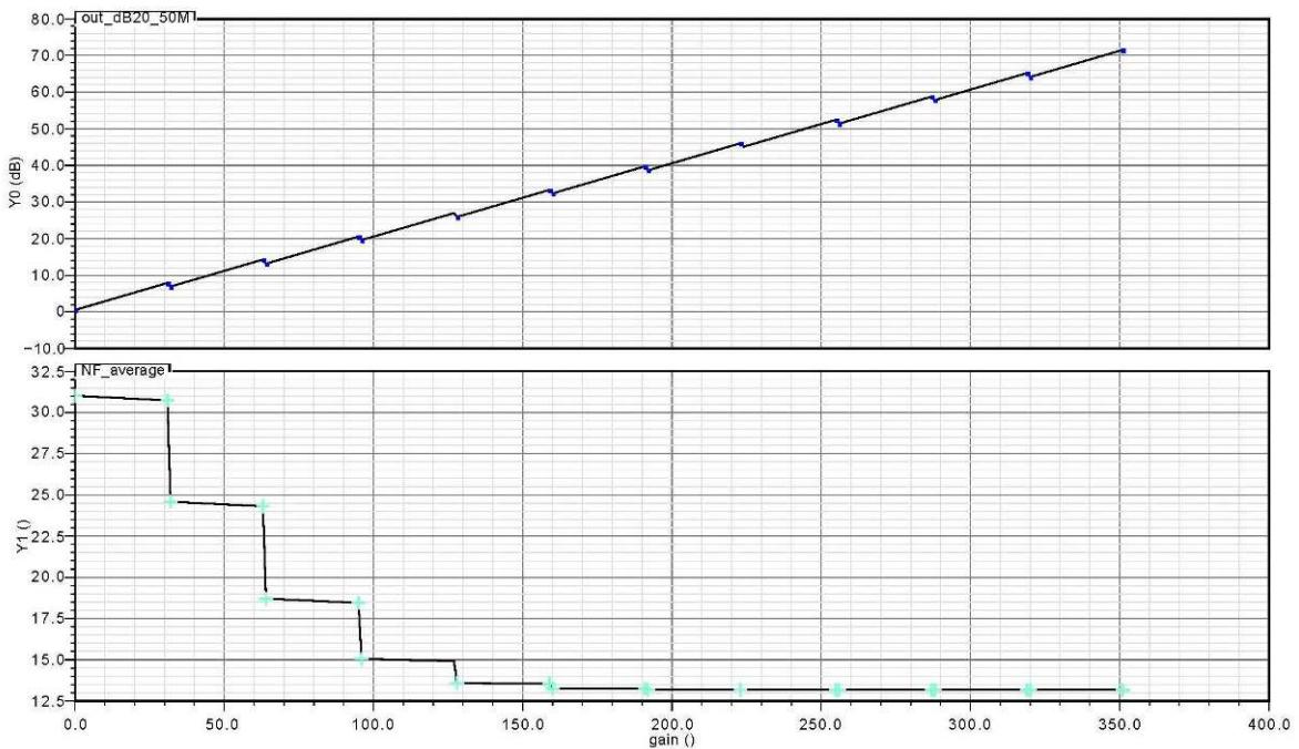
Figure 3: Gain characteristics, NF over code IFA
