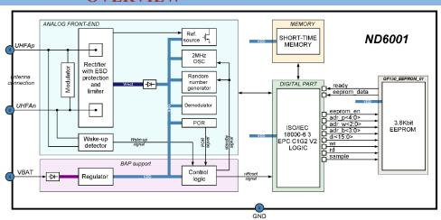
anti-collision protocol based on internal random number generator according to EPC standard. ND6001 supports all EPC C1G2 mandatory commands. The chip contains an embedded 3.6Kbit EEPROM organized in 4 banks.
