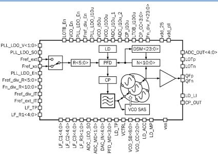
compensation VCO gain variation within band and keep loop parameters constant. Integrated low-pass loop filter has adjustable values of resistance and capacitance for tune loop and get best phase-noise performance. IP technology: TSMC CMOS CRN65LP.
