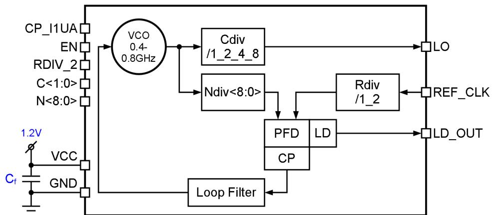
detector (LD) and programmable clock divider to obtain a required output frequency. Output frequency is calculated by formula:  $F_{LO} = (F_{ref}*N)/(R*C)$ . Output signal is CMOS compatible.
