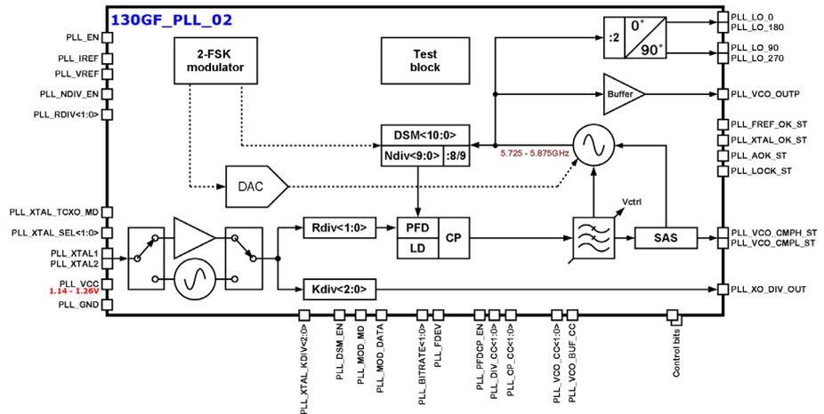
Quadrature former is intended to generate differential output signals with phase shift 90°, coherent to input signal.
