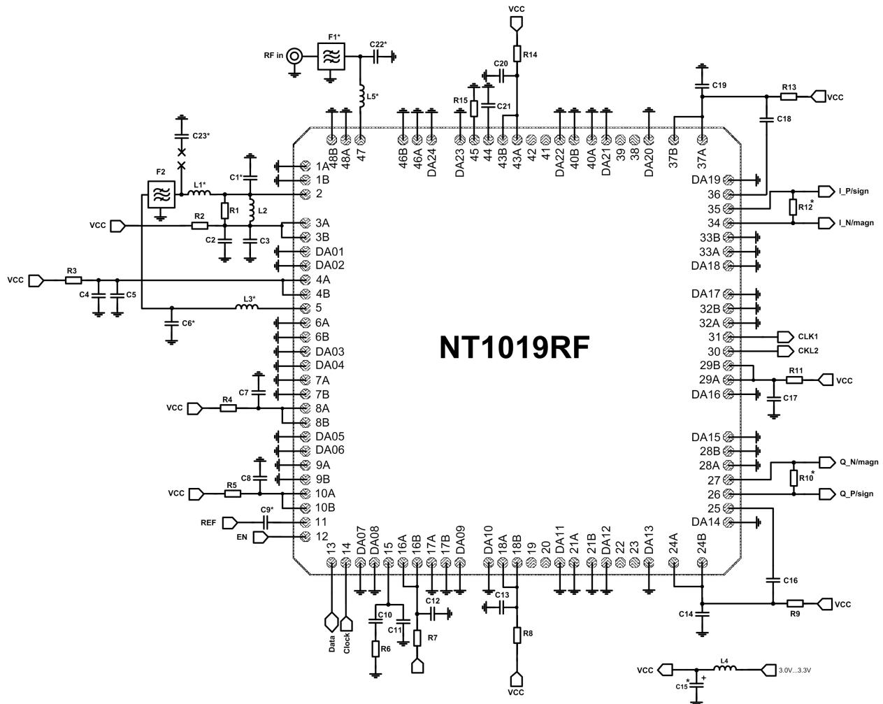
Figure 1: NT1019RF application circuit.
