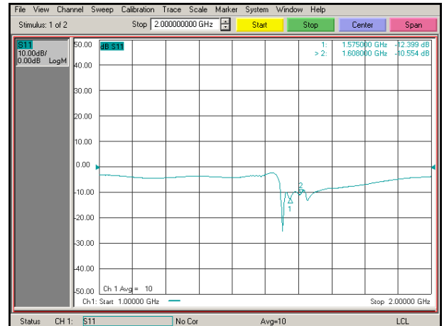
Figure 10: Active antenna input matching.
