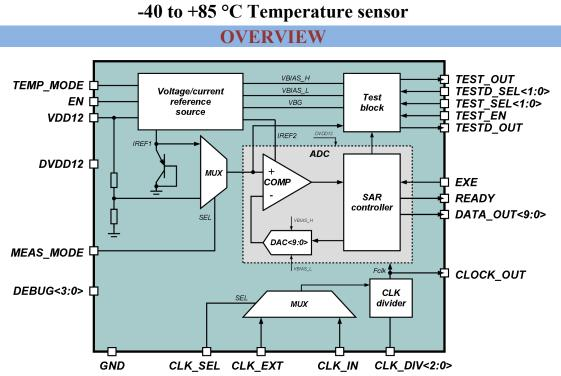
130GF\_TS\_01 is a Temperature detector with unique solution intended to continuously monitor IC temperature. It converts temperature between -20°C and +45°C to a 10-bit digital word with  $\pm 0.5$ °C accuracy,  $\pm 0.3$ °C accuracy for temperature range +30°C  $\div$  +45°C and  $\pm 1$ °C accuracy for temperature range -40°C  $\div$  +85°C. Temperature detector consists of temperature sensor unit, voltage and current reference block, ADC and test block.
