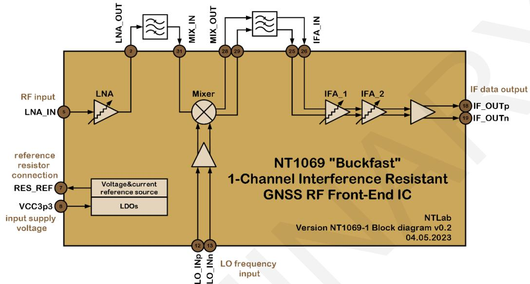
Figure 4.1: NT1069-1 “Buckfast” Block diagram
